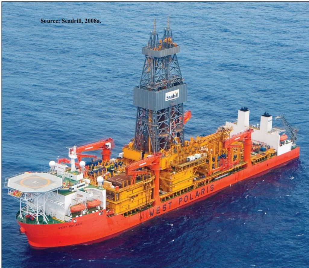
Dual activity derrick on the 6 th generation West Polaris drillship built in 2008.
